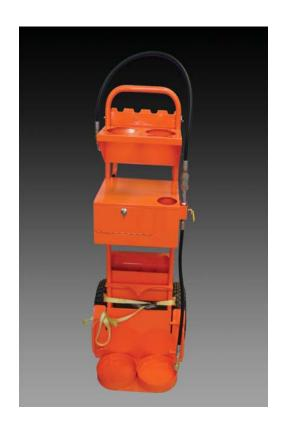
to fill two units at the same time. There is a locked compartment for tools, cleanup materials and filling funnel. A fixed bottle serves to drain the funnel after use and to store excess filling solution. A built-in waste basket will store waste cleaning materials.
