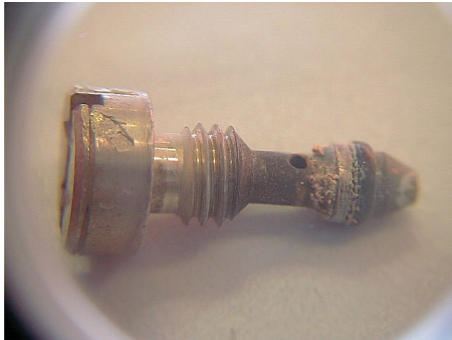
Photo 8. Valve Needle Deposits
