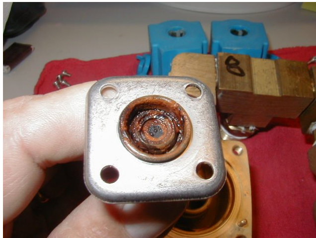
Photo 7. Solenoid Plunger Deposits
