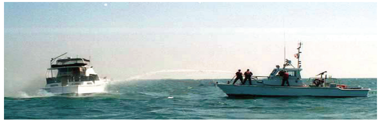
WRSS uses existing ship firefighting system.
