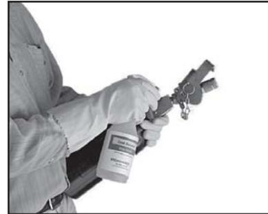
8. Remove the funnel from the plastic storage bag and place in top of bottle. Remove cap from one bottle of refill solution and carefully pour into the cylinder using the funnel. Allow funnel to drain thoroughly before removing it from the bottle. When done, place the funnel back in the storage bag. Properly discard empty bottle using standard operating procedures for OC chemicals.
